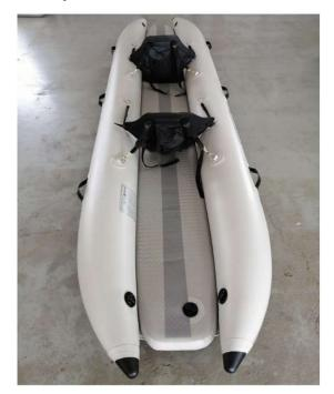
**Step 1:** Remove the hose set from the carrying bag and lay it spread out on a flat surface. Check that the valve plugs are in the filling position.
